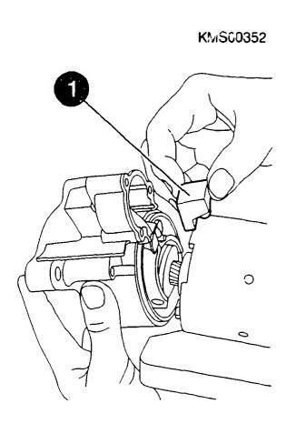
Disassembling overrunning-clutch drive and planetary gear train
